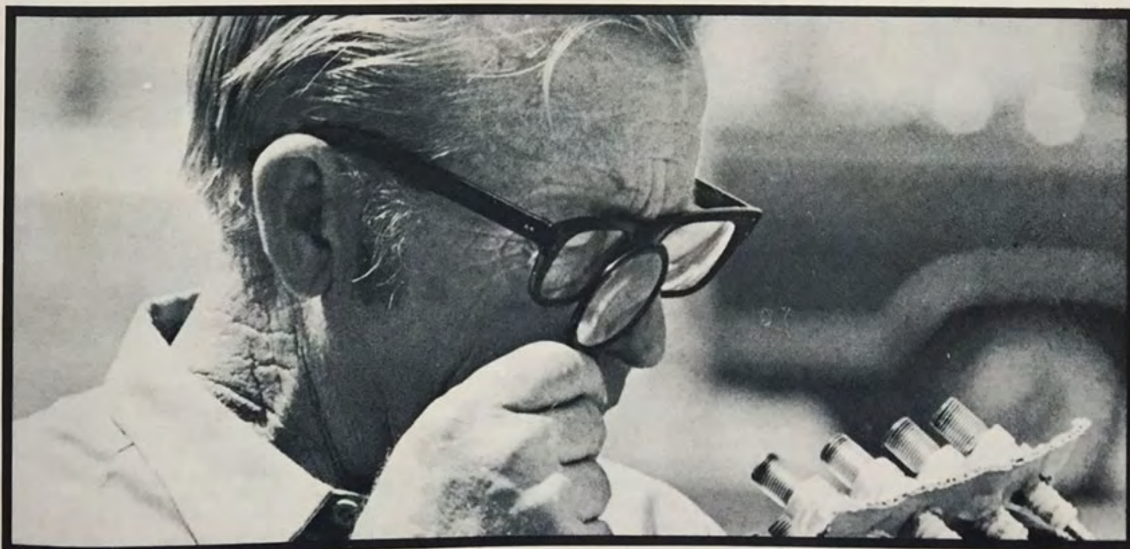
Owens is a meticulous engine builder and tuner. Here he checks spark plugs for clues to the stage of tuning the Dodge Hemi is in. His careful work contributed to Buddy Baker's win at this year's Southern 500, the most prestigious of stock car races.
